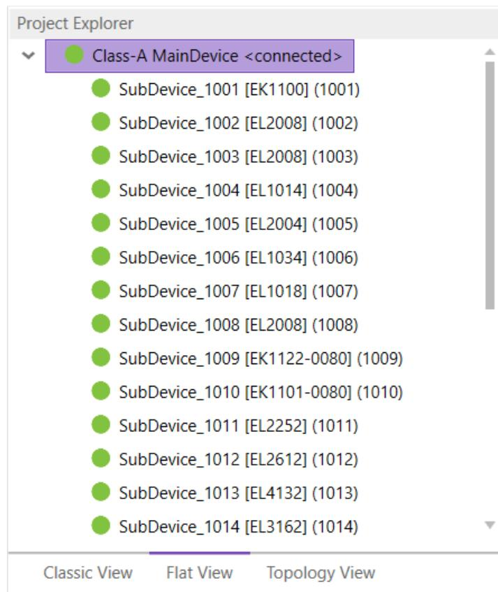
This view shows all SubDevices in a flat list, as they are connected in the EtherCAT network.
