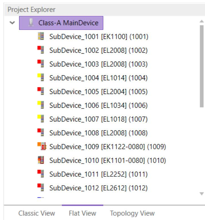
This view shows all SubDevices in a flat list, as they are connected in the EtherCAT network.
