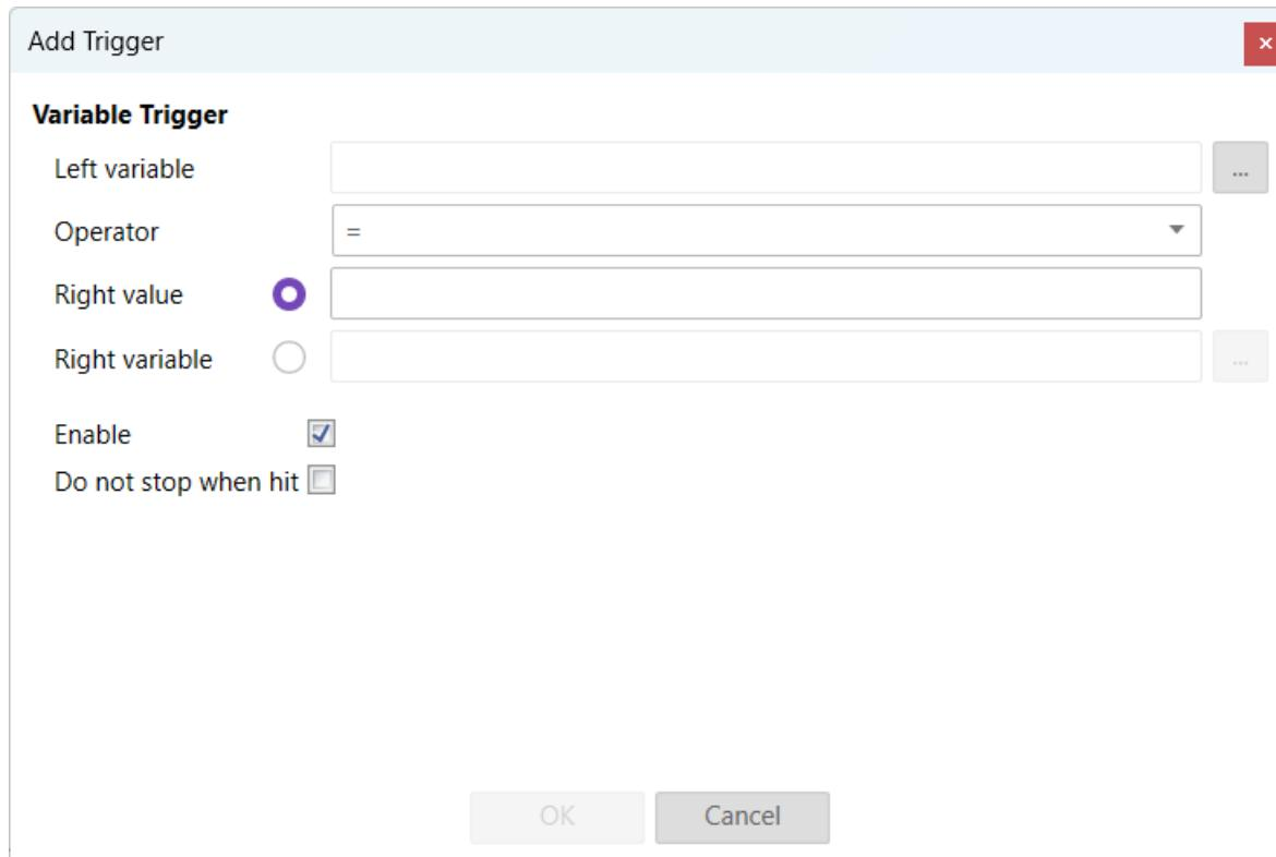
The user can select variable which should be compared and the select if he wants to compare with a value or another variable. With enable the trigger can be enabled and disabled.
