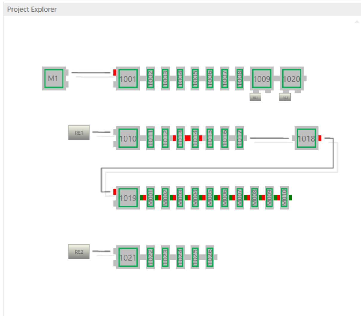
This view shows a graphical tree of all SubDevices, as they are connected in the EtherCAT network.
