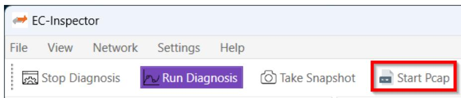
It is also possible to record a pcap backtrace file. When EC-Inspector is in pause mode (e.g. from a trigger condition) the user can capture the last 64 frames via the backtrace button in the toolbar.
