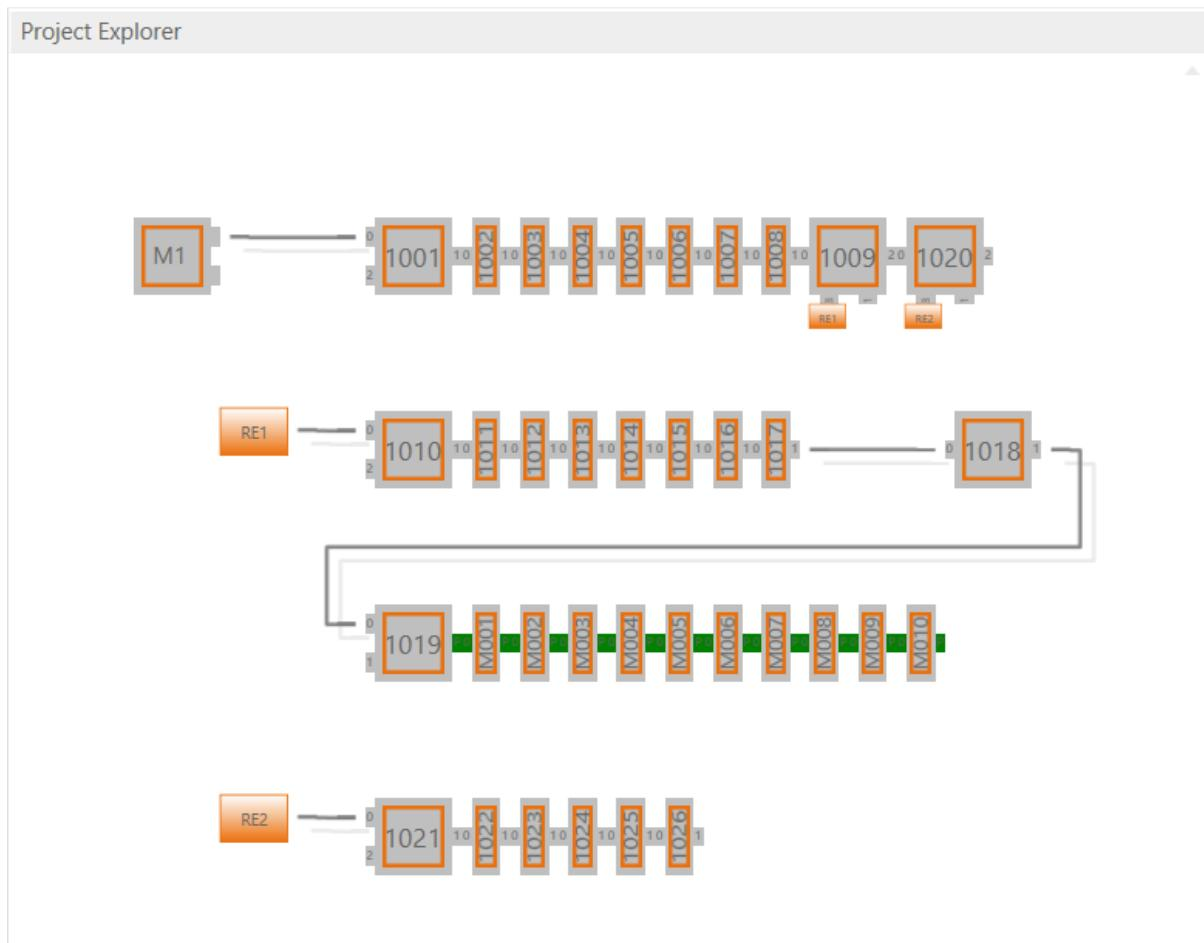
This view shows a graphical tree of all SubDevices, as they are connected in the EtherCAT network.
