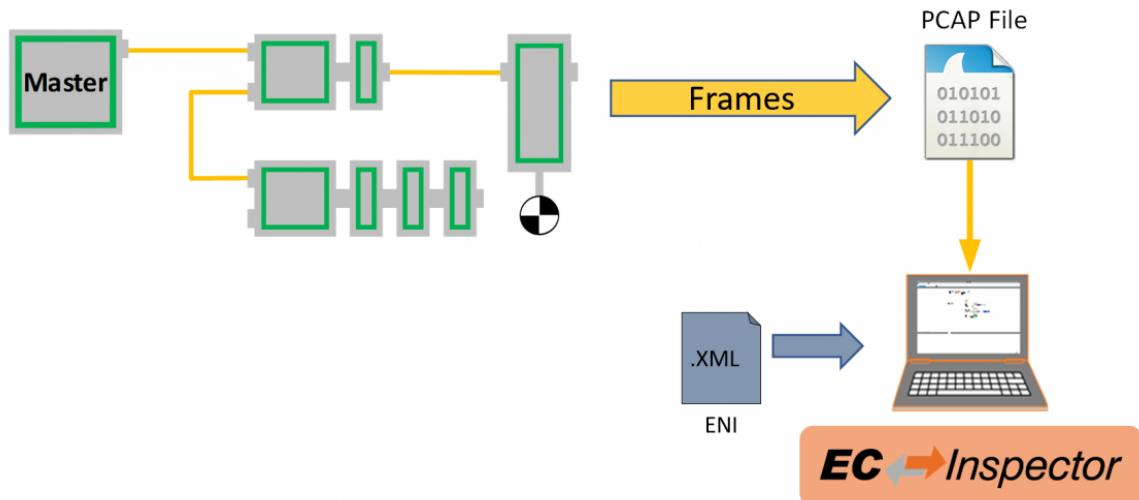
Therefore a wireshark have to be captured and saved as pcap or pcapng. Then it can be selected in the starting view of the EC-Inspector. Also the ENI file has to be selected.
