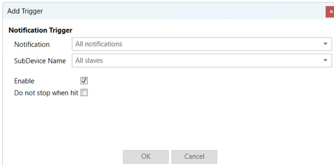
The user can select which notification should be triggered. He can also select for which SubDevice the notification should be triggered. Default is "All SubDevices". It is also possible to trigger all notifications for all SubDevices.
