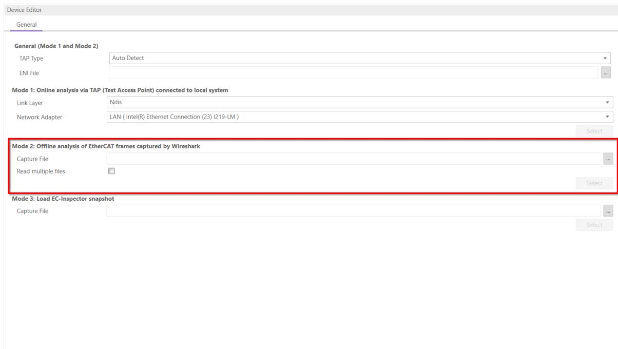
It is also possible to read multiple files. Therefore the pcap files have to named like that: name.00000.pcap.
